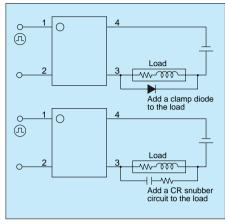
2) If spike voltages generated at the load are limited with a clamp diode and the circuit wires are long, spike voltages will occur by inductance.
